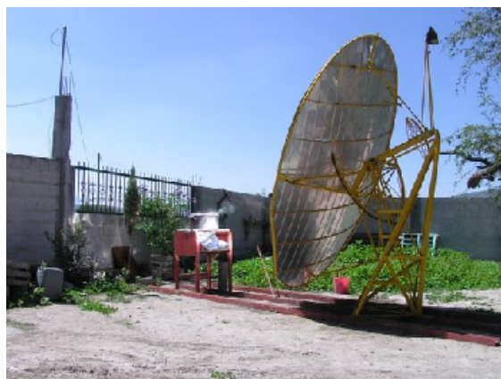
Picture 9: testing the 8m 2 Scheffler Reflector
