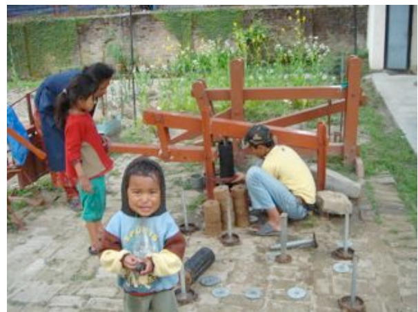
Fig.10 Making biomass briquettes in press
