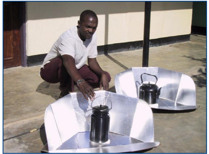
Solar water pasteurization using the CookKit
