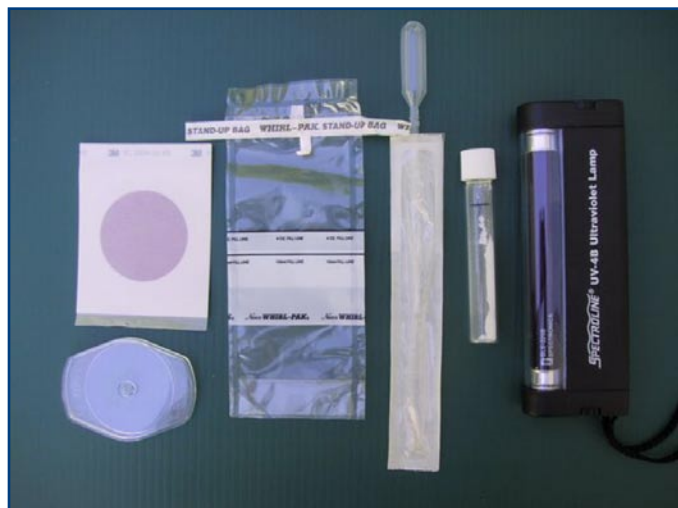
Contents of Portable Microbiology Laboratory
