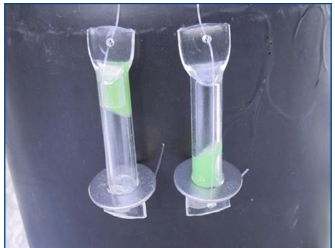
Reusable Water Pasteurization Indicators (WAPIs)
