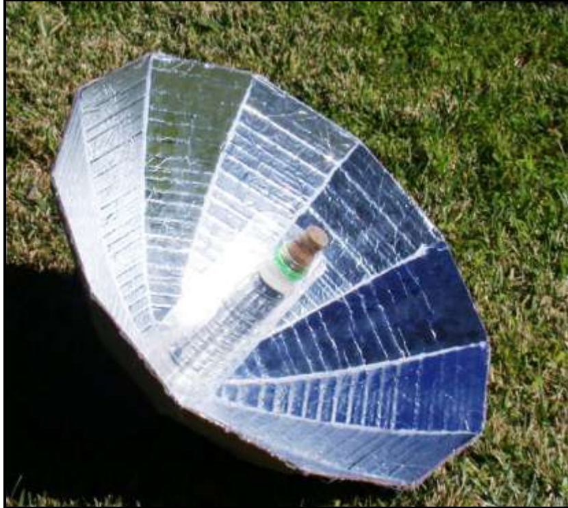
Figure 3. View of the solar water boiler assembly in use
