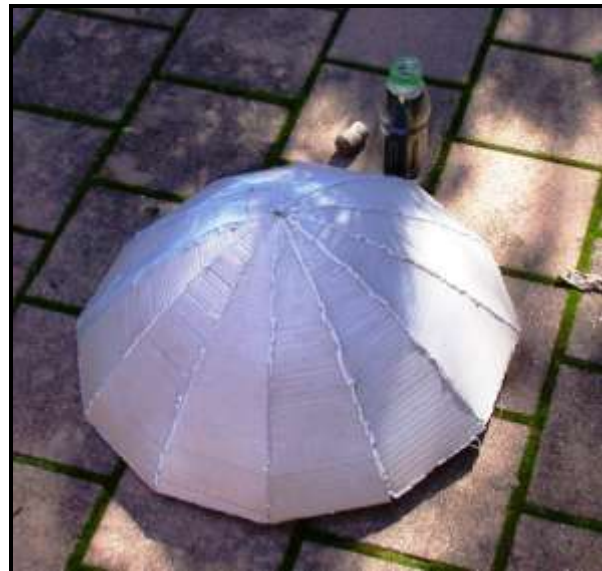
Figure 2. View of the completed parabolic reflector and insulated water bottle.
