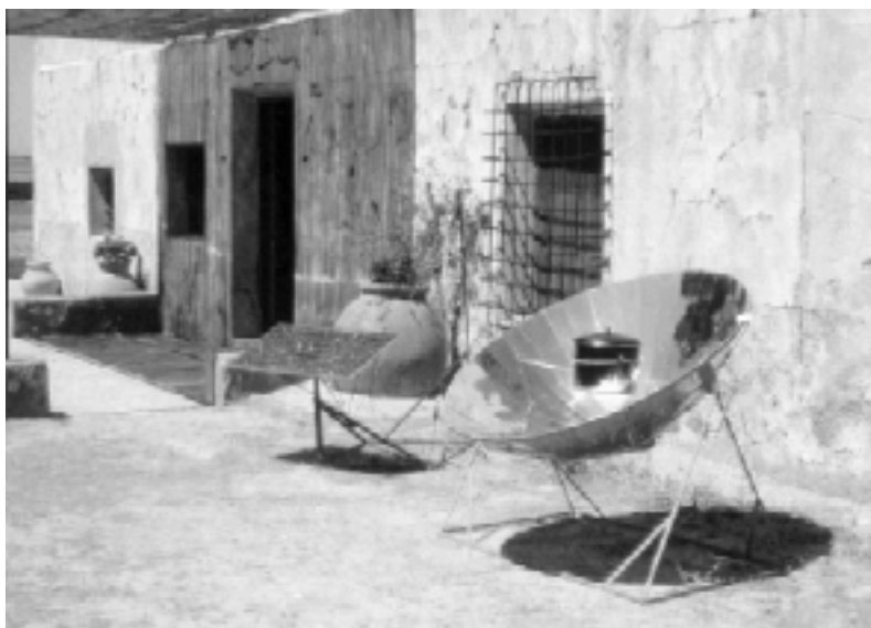
Fig. 3: Solar cooker SK12 and PV-panel for decentralised energy supply
