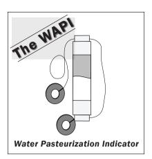
Disease-causing organisms in water are killed by exposure to heat in a process known as pasteurization. Boiling is often recommended to achieve pasteurization. However, contaminated water can be pasteurized at temperatures well below boiling, saving time and fuel. Water heated to 149°F (65°C) for a short period of time is free from microbes, including E. coli, Rotaviruses, Giardia and the Hepatitis A virus.
