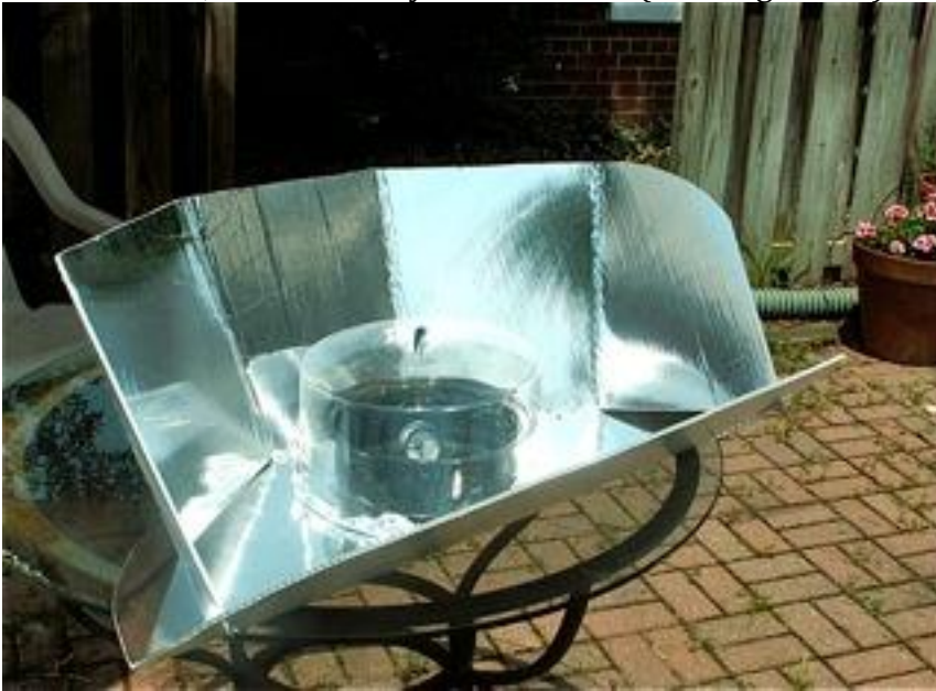
5. Water-proof, plastic flute board (Solar Clutch) a black metal pot with no-lid and a thermometer, under an acrylic cake dome (not a tight seal)--250 F after 40 minutes.
