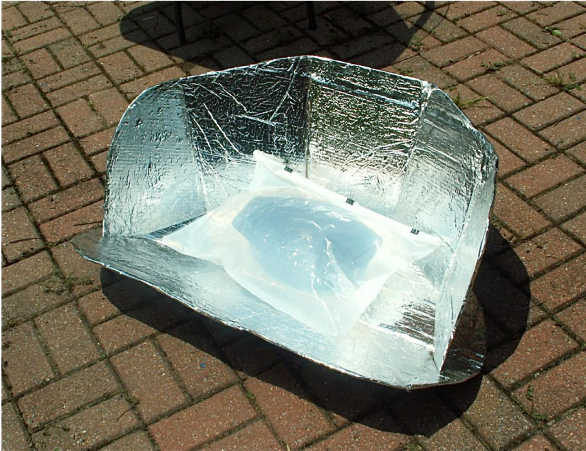
7. My homemade cardboard and aluminum foil solar cooker with Beacon Converter plastic bag (slightly milky plastic) rolled and sealed with metal binder clips, using a black metal pot with no-lid and a thermometer -- 200 f. after forty minutes.
