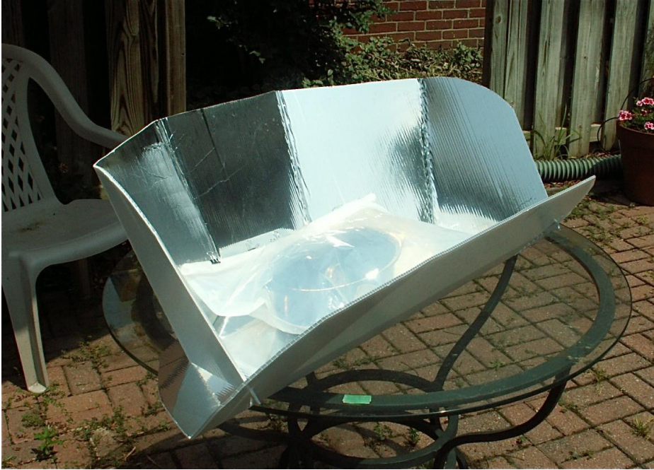
7. My homemade cardboard and aluminum foil solar cooker with Beacon Converter plastic bag (slightly milky plastic) rolled and sealed with metal binder clips, using a black metal pot with no-lid and a thermometer -- 200 f. after forty minutes.
