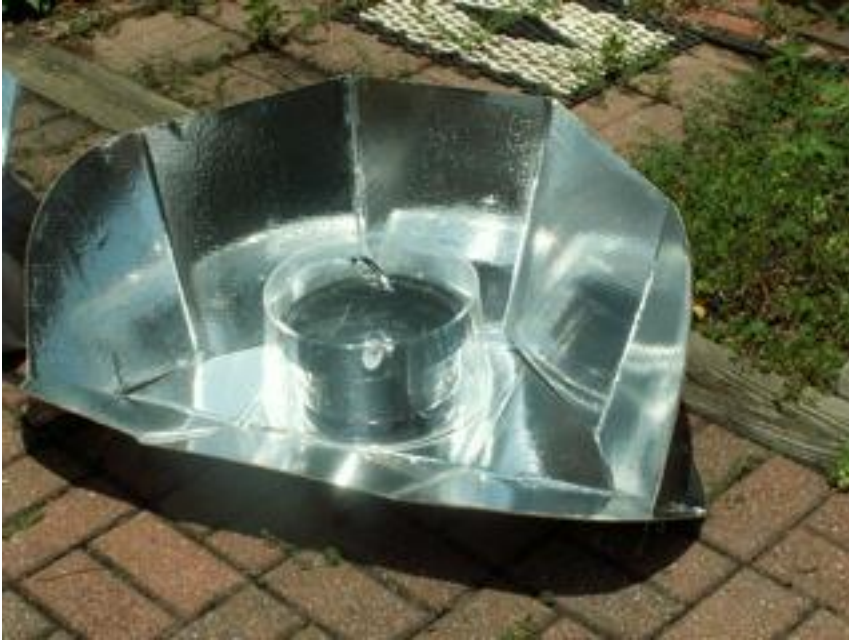
5. Water-proof, plastic flute board (Solar Clutch) a black metal pot with no-lid and a thermometer, under an acrylic cake dome (not a tight seal)--250 F after 40 minutes.
