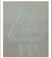
Looking a bit further on these containers I also observed the recycle symbol with the number 5 on it. After researching a bit more I found it to be Polypropylene in composition just like the autoclave bags we were using for solar cooking. I then found a large container of this same recyclable material and found it works great for solar cooking too.
