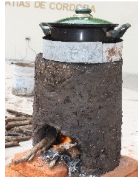
Rocket stove One-piece mud and dry grass
