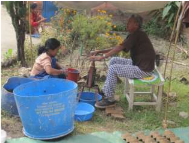
Leprosy patients couple and blind man pressing briquettes from biomass waste
