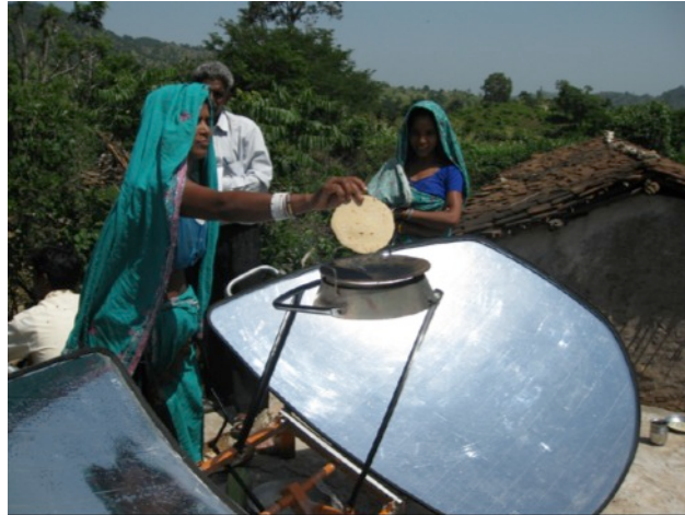
Figure 2: Namaste solar cooker being used to cook roti
