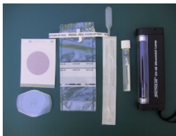
Water testing items: E. coli Count Petrifilm & spreader, Whirl-Pak, sterile pipette, 10 ml Colilert test, UV light
