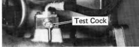
Fig. 3-3 - Low Water And Crankcase (Oil Pan) Pressure Detector
