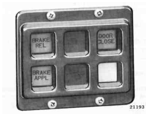
Fig. 2-19 - No. 2 Indicating Lights Panel
