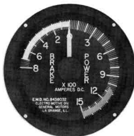
Fig. 2-20 - Load/Brake Current Indicating Meter
